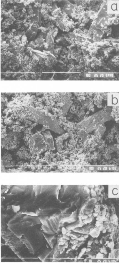
Fig. 4. Electron micrographs of: (a) crystals of the cured paste (refer Fig. 3), white line = 10 \mu\text{m} ; (b) agglomerates of active mass, white line = 100 \mu\text{m} ; (c) broken 4\text{PbO}\cdot\text{PbSO}_4 crystal, white line = 10 \mu\text{m} . (Taken from ref. 12.)
